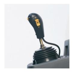
Low Effort Operation. Hydraulic joystick controls provide ease of lift and tilt functions. A single joystick is standard. An integrated directional control switch on the joystick provides easy operation and enhanced productivity. A two lever control is optional.
