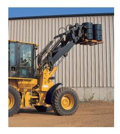
Parallel Lift Loader Linkage. The IT28G's 8-bar parallel design linkage keeps work tools such as forks level throughout the range of lift without adjustment by the operator. Superior load control is provided by more tilt capacity than lift in all positions. Long lift arms, tall front tower and high pivot points offer more height and reach than conventional loaders.
