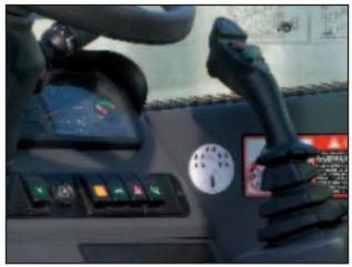
Single lever manipulator electro-hydraulically controlled. 9 functions provide complete control of all operations. Proportional control of arm extension provides maximum precision in load positioning.
