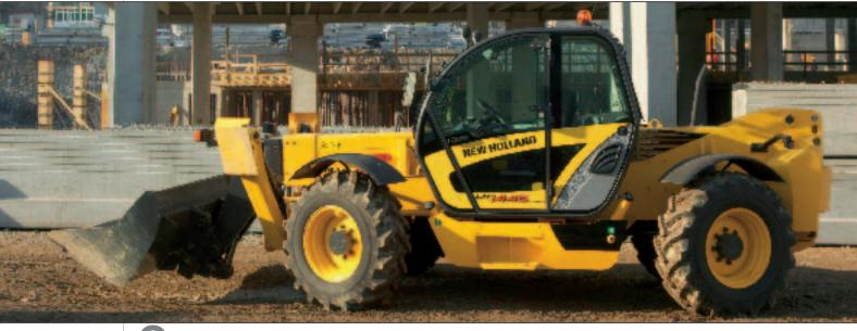
Ustanding steering radius (3.89 m) for working even in the most restricted areas. 4 wheel steering with 3 positions:
