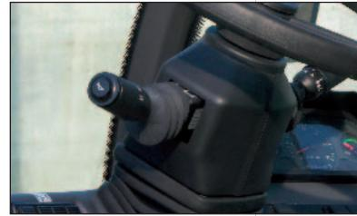
he transmission, PowerShift type 4+3 speeds, provides excellent precision in approach and positioning operations. High transfer speed: 35 km/h.
