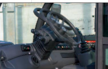
he continuously adjustable tilting steering column provides in the standard version a full range of operator's adjustments.
