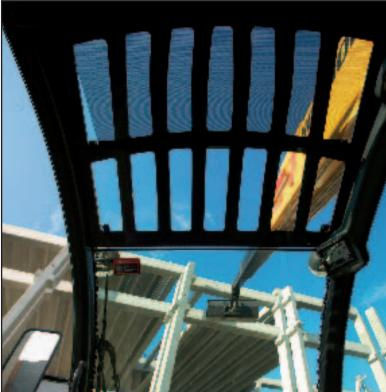
Gab door opens to 180° and secures at the fully open position. The door is constructed in two sections to enable the upper section to be opened independently.
